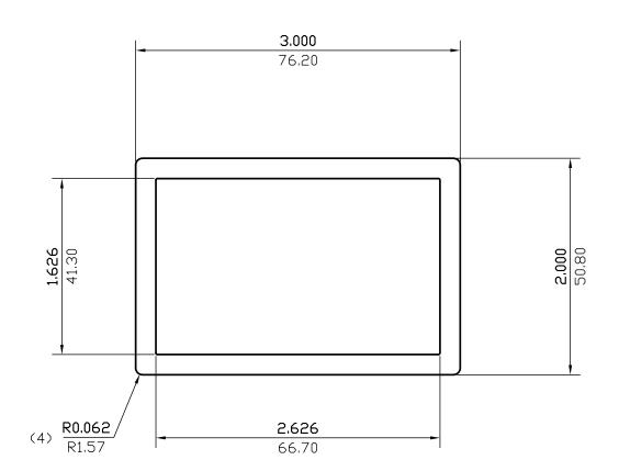
0.187(4.75)WALL THICKNESS EXCEPT AS SHOWN DATE REV DESCRIPTION BY 03/15/23 REMOVED ALLOY NDZAL мм.<sup>2</sup> 1114.211 1.727 IN.<sup>2</sup> EST.AREA EST.AREA 3.084 2.072 EST.WT. LBS/FT. EST.WT. KG/M. 18.372 466.644 EST.PER. MM. EST.PER. 9.894 251.3 OUT PER. MM. OUT PER. 3.555 90.302 C.C.D. C.C.D. FINISH M/F ALLOY FACTOR 9 SCALE 1:1 DWN BY L.G.DATE 01/03/2008 CKD BY
